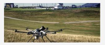
Equipped with an Orion semi automated tethered drone, Delta Drone provided persistent and safe flight missions during the competition. The live imagery from its day/night camera was broadcasted to the main control room, providing situational awareness, crucial for crowd monitoring, quick decisions making and rapid response.
