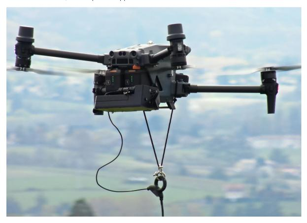
The onboard module allowing the tether power supply weighs only 500g and is easily fixed at the back of the drone. It offers a continuous power of 1000 Watts, allowing hours of flight at 70 meters without interruption, and resists temperatures between -20°C and +50°C. It also allows the operator to quickly switch from free flight mode to captive flight mode.
