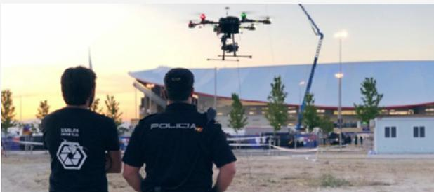
UMILES Global Solutions tethered their U06 drone to the Safe T station to be able to stay airborne during the entire mission. Two pilots oversaw the flight: one for the drone, and one for the camera. UMILES was allowed to fly in controlled airspace by the AESA and UNAIREs, the tether system being a reliable mitigation and a safer solution preventing all risks of fly away.
