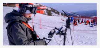
After a quick setup the station was powering the drone and streaming footage to SVT and the 700 Million viewers. With a Paralinx system reaching up to 600 meters, full HD images of 1080p and 50fps, with 0,1 seconds of latency were sent by fibre to a TV control center after being converted from HDMI/SDI to LAN/IP. The M600 was deployed up to 5 hours per day at temperatures reaching -15°C.
