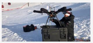
Aerocam tethered its DJI M600 with Elistair Safe-T station to increase the UAV autonomy for the 5 days of competition, but also to secure the drone's flight area and ensure the safety of the crowds. All equipment (Safe-T, drone, generator) fitted on a sled and 2 snow mobiles to climb the 1000m slopes, where Aerocam built up a start and landing surface to compensate the slope of the ground.
