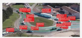
The tethered uav was strategically positioned ahead of the traffic, providing extensive coverage of the zone of interest. Data transfer was securely facilitated through the micro tether and directly displayed in real-time on the video monitor. A total of 7 826 vehicles were detected across 5 designated gates, with an average speed of 33 km/h.
