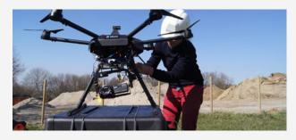
The drone was equipped with a digital Sony PJ 810 Full HD video handy-cam with a zoom x3. Tethered to an Elistair Safe-T station it performed a non-intrusive static flight for 3 hours at heights of up to 70m. A 50m radius zone was marked beneath the drone to ensure clearance from populated areas and mitigate potential hazards.
